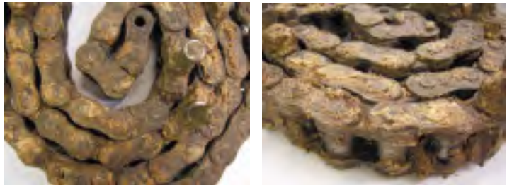
Hardened shell inhibits the passage of lubricant to the bearing area.
