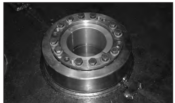
Custom Engineering Class Sprocket Assembly With Shrink Disc to Clamp Hub to Shaft.
