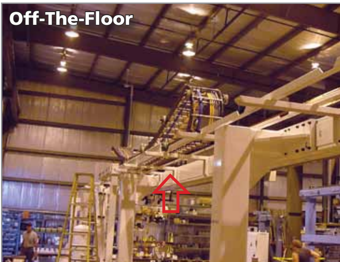
Nylon polymer cable and hose carrier system with elastically lowered mounting height using RollerGlide KS technology to extend travel length capabilities.
